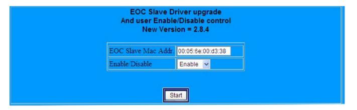
Figure 4.5.2.2.1 HPNA driver Upgrade and user speed control for Slaves
