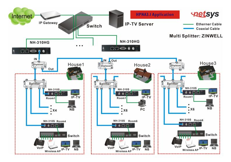
Figure 3.2 NH-310HG/S connection diagram-2
