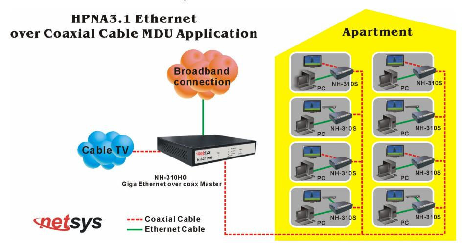
Figure 3.1 NH-310HG/S connection diagram
