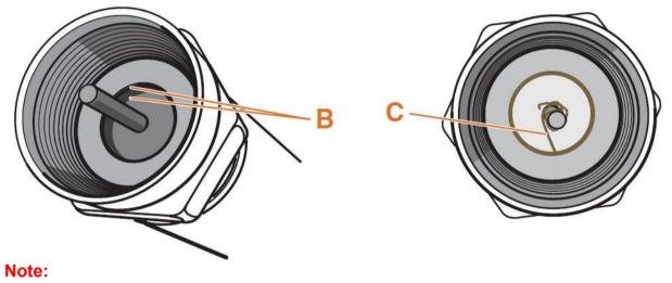
We recommend use RG59 75ohm coaxial cable to establish HomePNA network.
