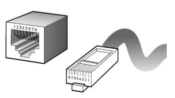
Figure A-1 Standard RJ-45 repectacle/connector
